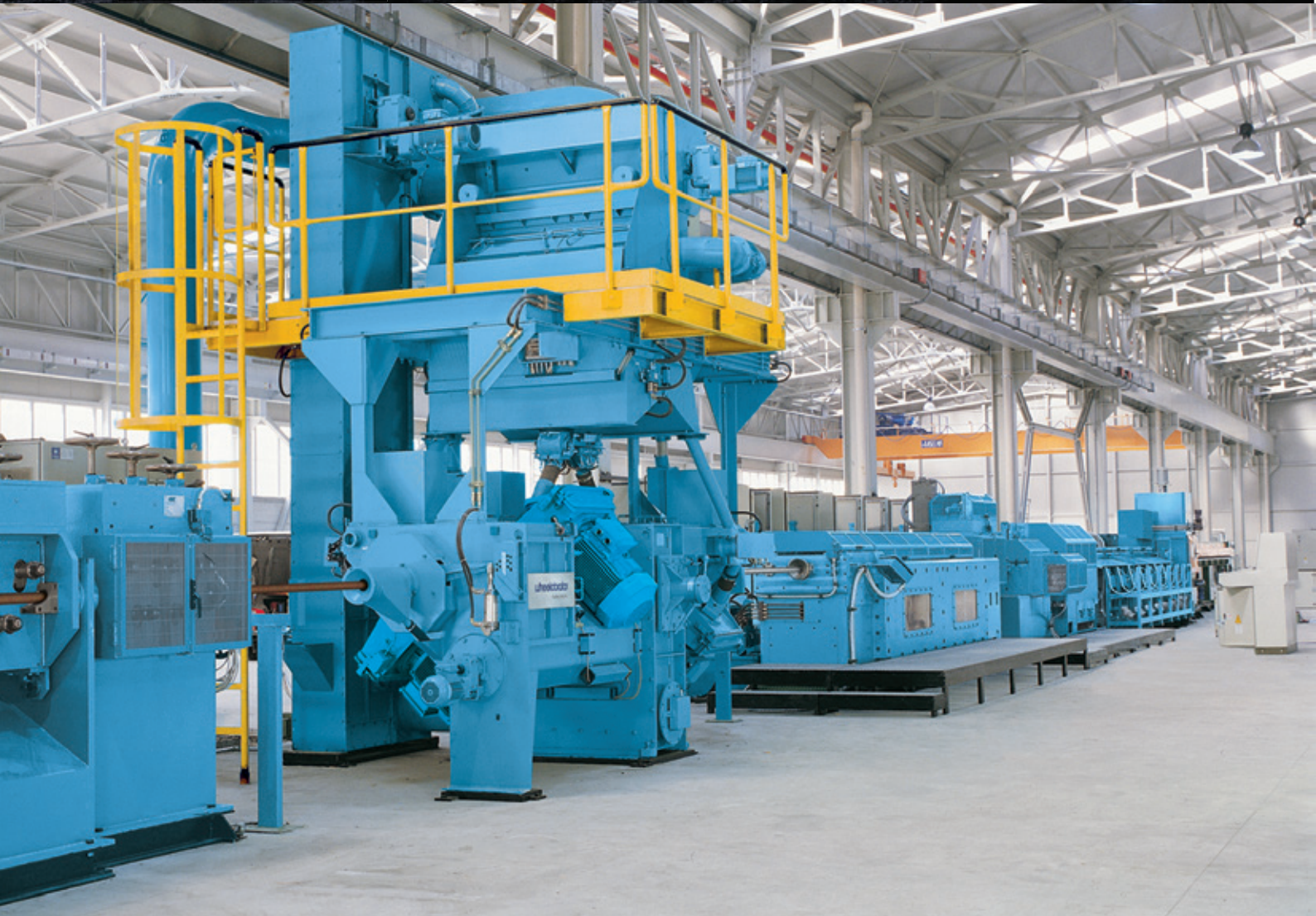
○ Wire descaling machine at SeAH Special Steel
