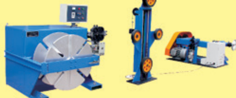
CQK550/700/850型主动放线成圈系统 CQK550/700/850 active pay-off /coiling systems
